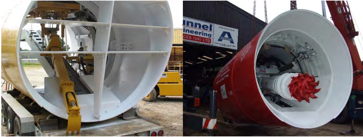
Figure 4: Example of a digger shield with partial face support and an excavator boom (left), and a digger shield with a road header excavator (right).
