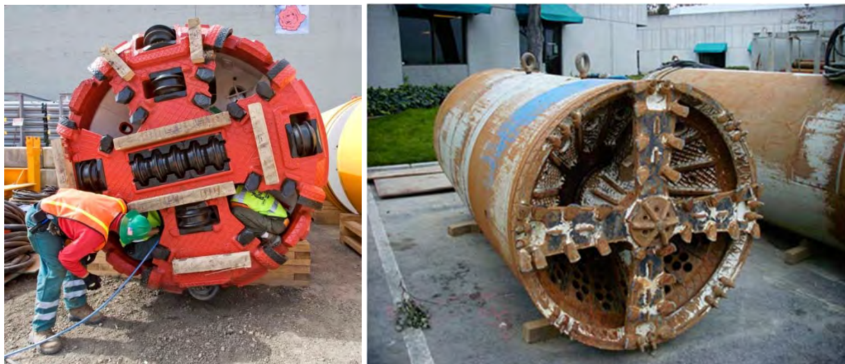
Figure 5: Example microtunnel boring machines. The cutter face is designed to suit the anticipated ground conditions.
